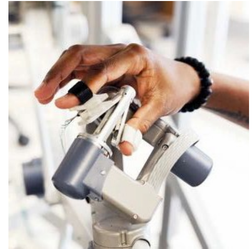
da Vinci Surgical System from Intuitive Surgical, Inc. (no programmable force feedback on gripper)
