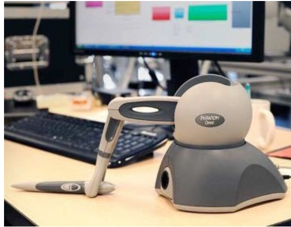
Phantom Omni/Touch from SensAble/Geomagic
