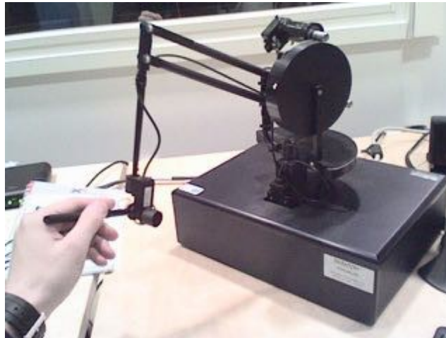
Phantom Premium 1.5 from SensAble/Geomagic
