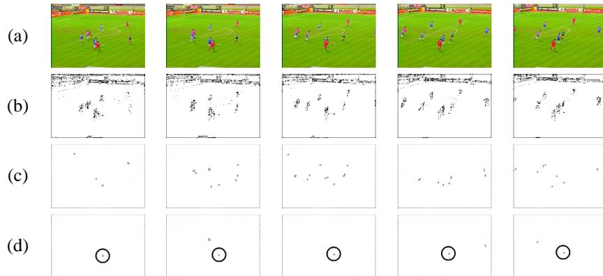
by detail pixels in the image, we proposed here a solution based on details removal using multiresolution filtering. A local analysis is then performed to detect candidate regions. A final interframe matching phase allows to isolate real small objects from noise and to track the objects along a video sequence.
