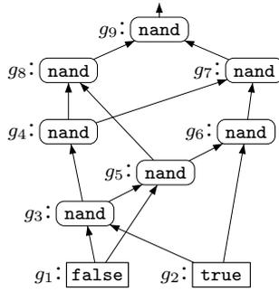
Fig. 2.  $\mathcal{C}$ , a Boolean circuit of **nand** gates.
