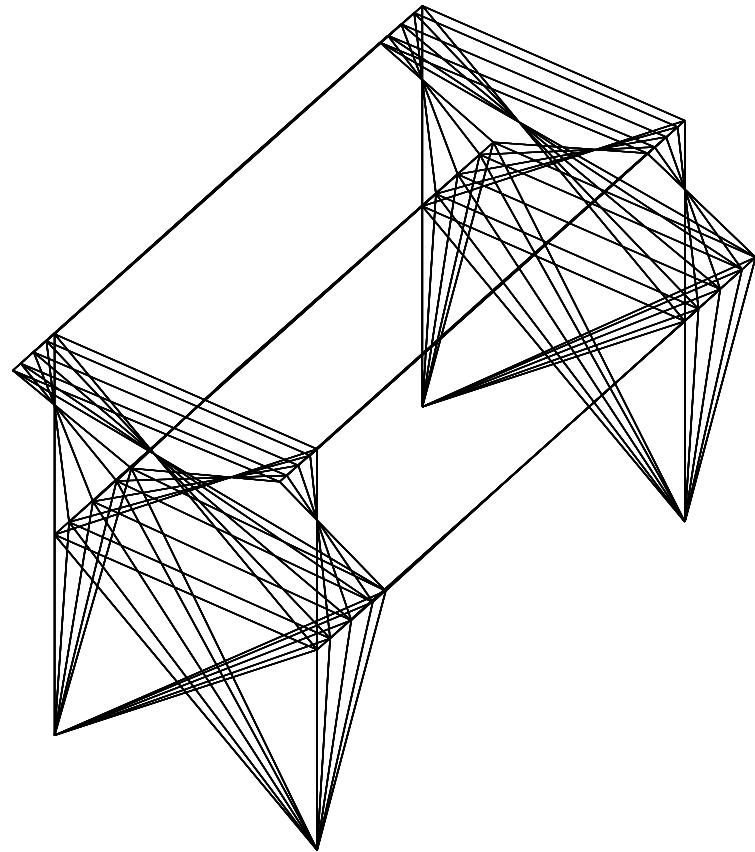
**Bending mode in X direction at frequency 10.8 Hz.**
