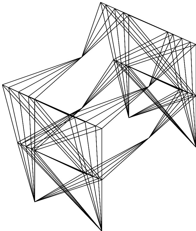
**Bending mode in  $Y$  direction at frequency 3.92 Hz.**
