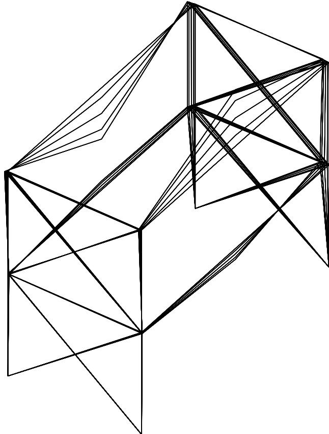
**Slab torsion in Z direction at frequency 17.7 Hz.**
