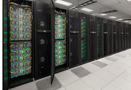
Stampede, U.S.A., #20 with \approx 5 Pflops 56 Gbit/s FDR InfiniBand Fat tree topology 6,400 \times (8 cores + 1 Xeon Phi)
