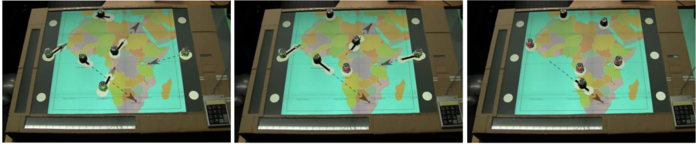
Fig. 7. Photographs illustrating how the robots move to reach their position by following lines displayed on the underlying screen. Arrows indicate the trajectories computed for each robot.
