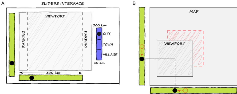
Fig. 6. (A) Sliders interface. For panning, users can move the viewport horizontally and vertically by moving two robots (black dots on the green areas) that represent the position of the viewport's center. Users can move the third robot in the zooming area (in blue) to select any scale between 30km and 300km. (B) Illustration of two successive sliders' and viewport's positions over the map.
