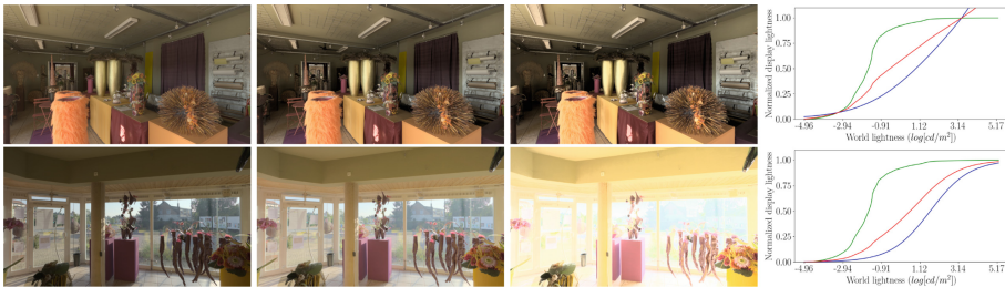
Fig. 7. Two opposite views in a same scene, a dark side (top) and a bright side (bottom). From left to right: the viewport TMO V(L_w(x, y), t) (blue curve), the combination of viewport and global TMOs L_d(G, V) (red curve), and the global TMO G(L_w(x, y)) (green curve). (Color figure online)
