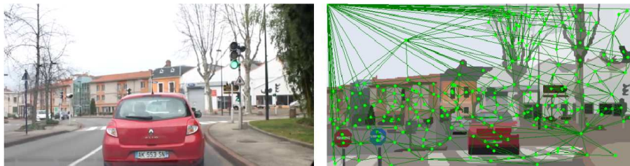
Fig. 1. Frame of a video and its corresponding RAG from a (static) segmentation.
