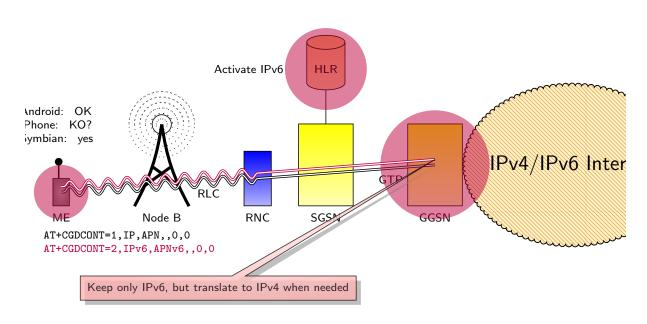
ME: Mobile Equipment, RNC: Radio Network Controller, SGSN: Serving GPRS Support Node, GGSN: Gateway GPRS Support Node, HLR: Home Location Register, GTP: GPRS Tunnelling Protocol RLC: Radio Link Control
