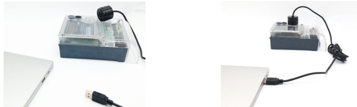
Fig. 13. Optical probe connected to the power meter (source: https://www.aliexpress.com/item/China-Manufacturer-DHL-free-Shipping-electricity-optical-meter-reading/32455842504.html?spm=2114.10010108.100009.1.6810cc24soIZC4&gps-id=pcDetailLeftTopSell&scm=1007.13482.95643.0&scm_id=1007.13482.95643.0&scm-url=1007.13482.95643.0&pvid=65873a85-f01b-4876-970d-b58b38041880 )
