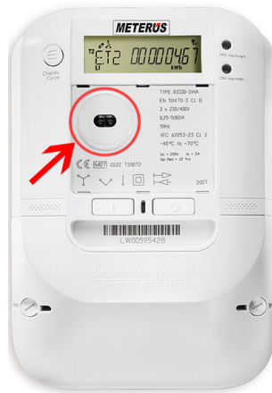
Fig. 12. A power meter with an optical port (source: https://nl.wikipedia.org/wiki/IEC_62056 )
