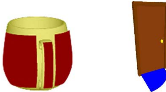
Figure 11: Interaction surface on a cup (dark areas where to place hands to pick it up) and influence surface of a door (area in front of the door to stay clear of) [Badawi07].
