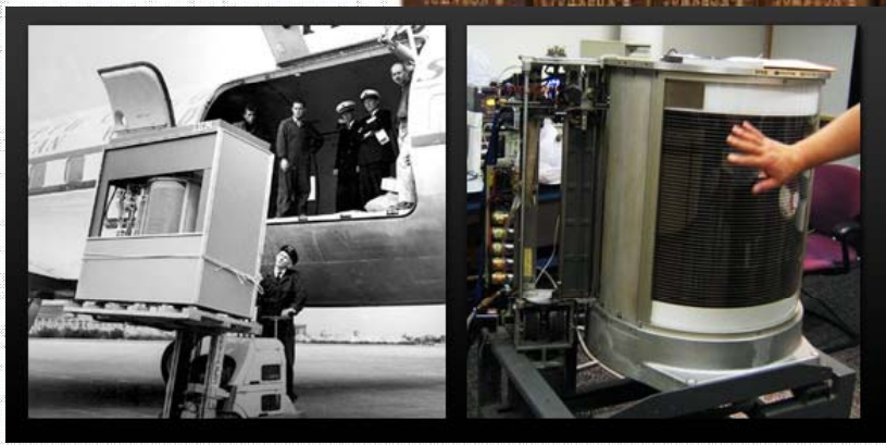
IBM Model 350, the first-ever hard disk drive. 5 Million Characters (5MB).
