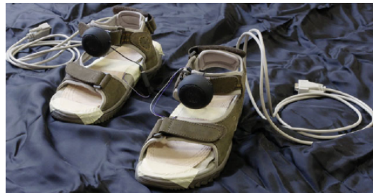
Fig. 10 Photo of the actuated shoes [76] with loudspeakers mounted on the top. The cable in the foreground interfaces the sensors in the shoes with the data acquisition unit.
