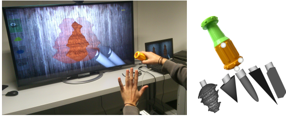
Figure 2: (Left) Collocated setup with the two hands: the left hand can select the tip using a panel while the right hand manipulates the Multi-tool through a generic real handle. (Right) Examples of interchangeable tips of our Multi-tool approach.
