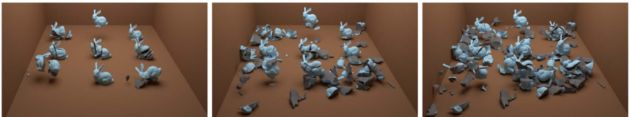
Fig. 13. Bunnies are dropped in three batches and fractured into 166 fragments and 435K triangles. The complete simulation runs at 24.5 ms per time step on average, with a maximum of 81.5 ms.
