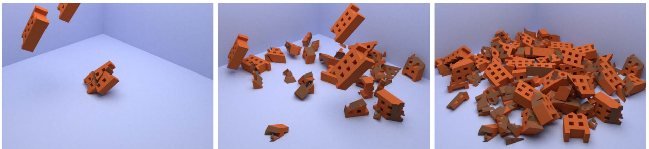
Fig. 14. Real-time demo of crashing bricks, totaling 156 fragments and 40K triangles. The complete simulation runs at 11.7 ms per time step on average, with a maximum of 29.5 ms.
