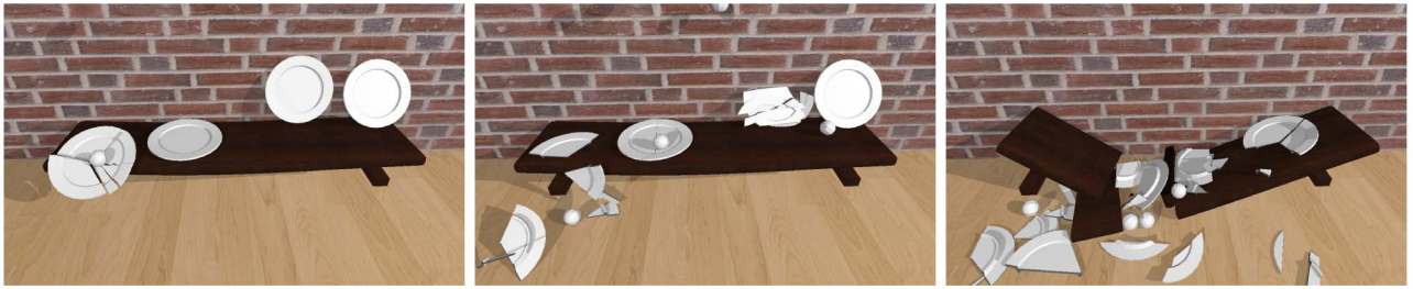
Fig. 1. Smashing plates . The user drops balls in real-time to smash the plates, and at the end of the simulation the scene consists of more than 45K triangles. The complete simulation runs at 7.4 ms per time step, on average, with a maximum of 13.2 ms.
