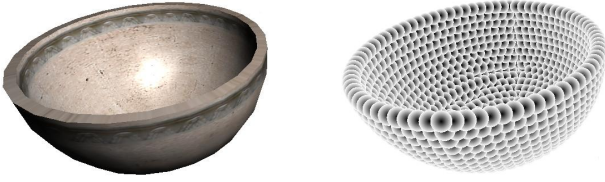
Fig. 3. Rigid body particle sampling. The mesh bowl (left) is converted into a set of particles (right).
