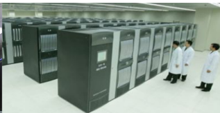
#2 Tianhe 2 3,120,000 cores 56 Tflops, 18MW
