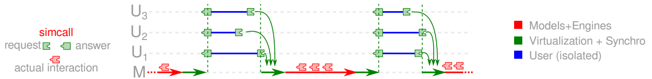
Figure 3.9 – Enabling Parallel Execution with simcalls for Process Isolation.
