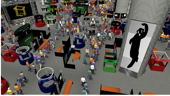
Figure 2: A simulation frame from the Trade Show Floor consisting of 1,000 agents. PLEdestrans computes collision free trajectories with many emergent behaviors at 31 fps.
