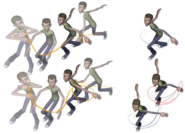
Figure 4: Global and local spaces. Top: Motion of the left wrist in the global space (left) and in the local space with respect to the shoulder (right). The local space reveals a simple backward swing of the arm followed by a larger forward swing. In this case, the local space permits a more intelligible display of the extent and orientation of the arching motion. Bottom: An edited motion (left) with a single stroke on the local space (right).
