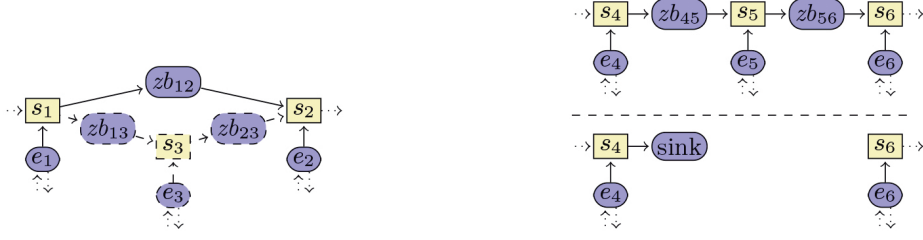
Fig. 6. Reconfigurations in the flood monitoring system: adding sensor s_3 , which requires connecting it to existing sensors s_1 and s_2 through new ZigBee connectors (left), and removal of sensor s_5 (right).
