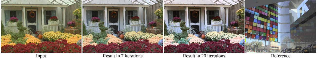
Figure 4. Results from applying cluster-based CAT algorithm. For this pair of input/reference images, CAT algorithm converges in 20 iterations. After the first 7 steps, the input image is already adapted to the reference illuminant. However, there is still a cast of the greenish input illuminant which is removed by the time the algorithm converges.
