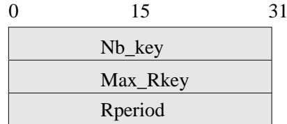
Figure 5: The KRI RR wire format.
