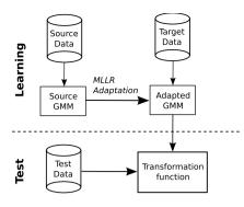
Figure 1: Architecture of the conversion system with source GMM adaptation to target data.
