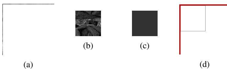
Figure A.15: Prediction of a luminance image block of size 64 \times 64 pixels via the selected H.265 function. The selected H.265 function, called DC, predicts each block pixel as the average of the neighboring pixels colored in red. Its index is 1.
