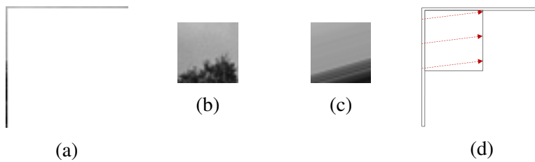
Figure A.9: Prediction of a luminance image block of size 32 \times 32 pixels via the selected H.265 function: (a) previously encoded and decoded neighboring pixels, (b) block to be predicted, (c) predicted block via the selected H.265 function, and (d) prediction sketch (the dotted arrows indicating the direction of propagation). The index of the selected H.265 function is 7.
