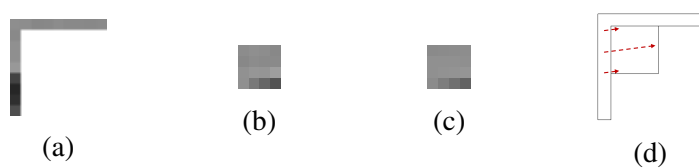
Figure A.3: Prediction of a luminance image block of size 4 \times 4 pixels via the selected H.265 function. The index of the selected H.265 function is 8.
