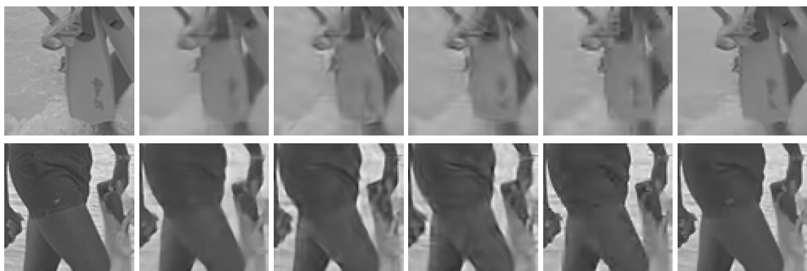
(a) original (b) orange (c) green (d) red (e) JPEG2000 (f) H.265 crops (0.179, 34.123) (0.120, 33.123) (0.124, 33.193) (0.153, 33.641) (0.178, 36.280)
