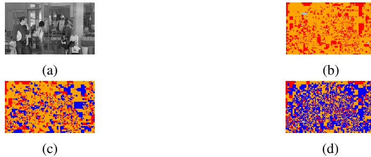
Figure C.3: Comparison of the three maps of intra prediction modes: (a) 832 \times 480 luminance channel of the first frame of BQMall, (b) map of intra prediction modes via H.265, (c) map of intra prediction modes via PNNS substitution , and (d) map of intra prediction modes via PNNS switch . For the three encodings, QP = 32 .
