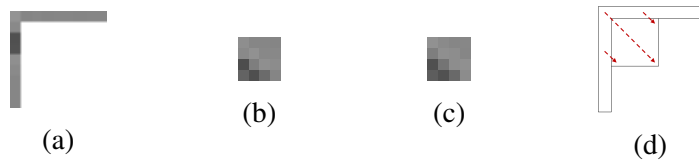
Figure A.1: Prediction of a luminance image block of size 4 \times 4 pixels via the selected H.265 function: (a) previously encoded and decoded neighboring pixels, (b) block to be predicted, (c) predicted block via the selected H.265 function, and (d) prediction sketch (the dotted arrows showing the direction of propagation). The index of the selected H.265 function is 17.
