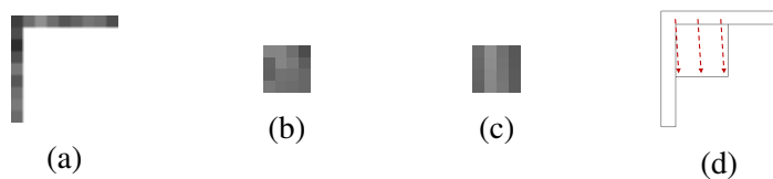
Figure A.4: Prediction of a luminance image block of size 4 \times 4 pixels via the selected H.265 function. The index of the selected H.265 function is 25.
