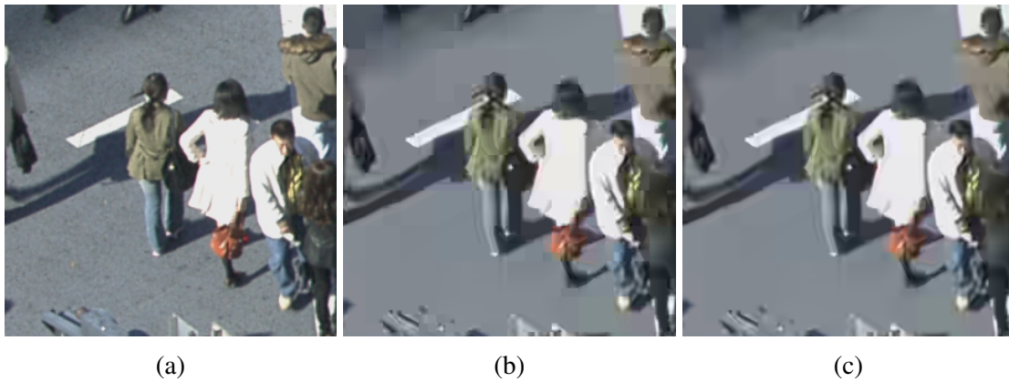
Figure 2.11: Visualization of blocking artifacts: (a) a 300 \times 300 crop of the first frame of PeopleOnStreet, (b) its reconstruction via H.265 with the DBF turned off, and (c) its reconstruction via H.265 with the DBF turned on. QP = 42 .
