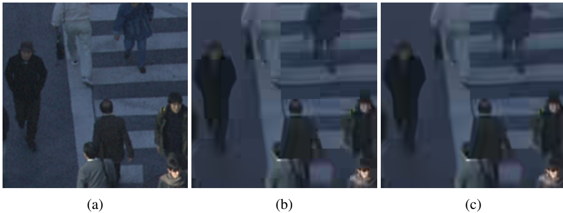
Figure 2.12: Visualization of blocking artifacts: (a) another 300 \times 300 crop of the first frame of the video PeopleOnStreet, (b) its reconstruction via H.265 with the DBF turned off, and (c) its reconstruction via H.265 with the DBF turned on. QP = 42 .
