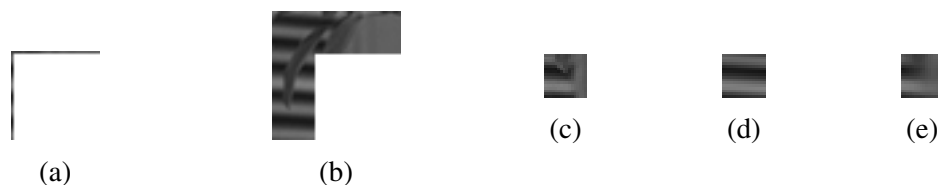
Figure 5.10: Prediction of a block of size 16 \times 16 pixels via the best H.265 mode in terms of PSNR and PNNS: (a) H.265 causal neighborhood, (b) PNNS context, (c) block to be predicted, (d) predicted block via the best H.265 mode (of index 11) in terms of PSNR, and (e) predicted block via PNNS.
