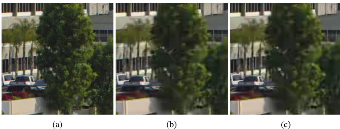
Figure 2.13: Visualization of blocking artifacts: (a) a 300 \times 300 crop of the first frame of the video Traffic, (b) its reconstruction via H.265 with the DBF turned off, and (c) its reconstruction via H.265 with the DBF turned on. QP = 42 .
