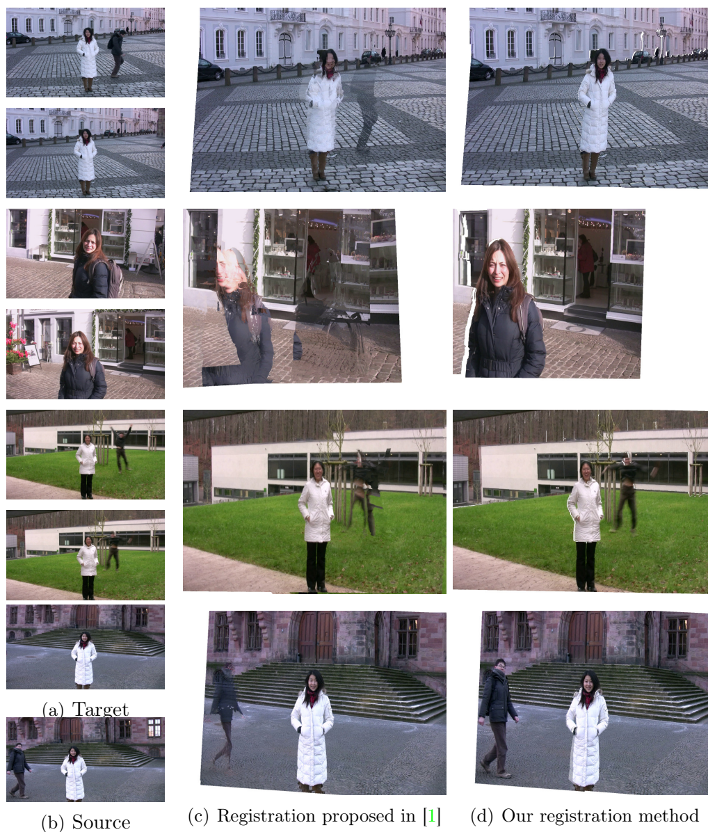
Figure 6.12: Comparison of registration quality with scenes having different types of camera motion. First row: slow rotation. Second row: fast view changes. Rows 3 and 4: small view change and zooming. (a) Target image. (b) Source image(to be registered to the target).
