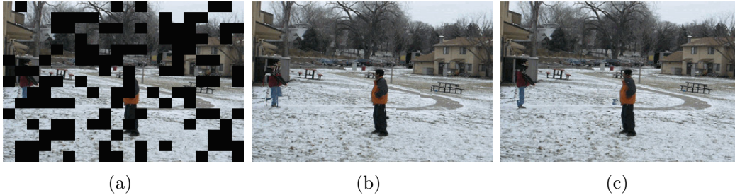
Figure 3.15: Performances of the proposed approach in the error concealment application. - (sequence Duo); (a) Image with 50% of blocks are lost (first column) (PSNR=9.01 dB); (b) image recovered using motion compensation (second column), (PSNR=28.26 dB); (c) image recovered using the proposed algorithm (third column), (PSNR=32.23 dB).
