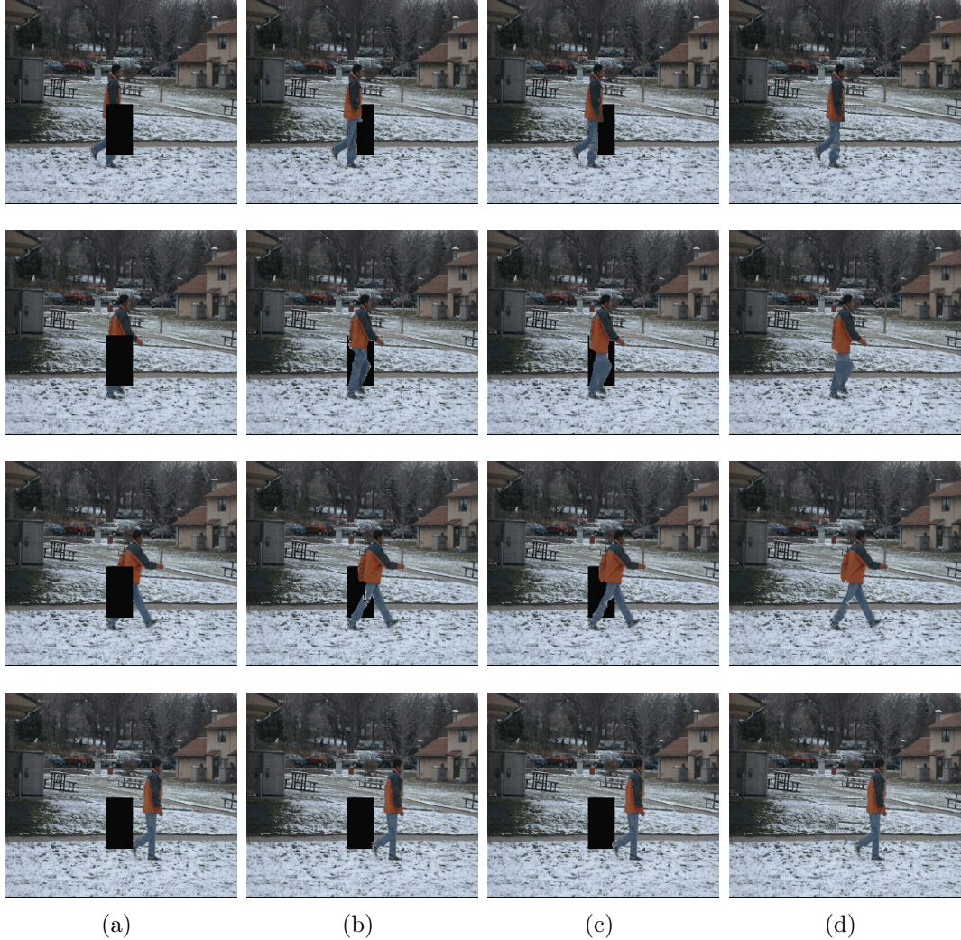
Figure 3.12: Impact of the neighbor embedding technique on inpainting results. - (sequence Man); (a) Original image + mask; (b) Moving object inpainted with the TM-based algorithm in [8]; (c) Moving object inpainted with the proposed approach; (d) Inpainted result with the proposed approach;
