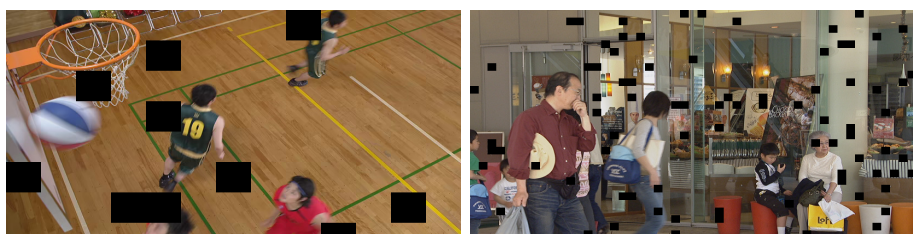
Figure 3.16: Test video sequences (BasketBallDrill and BQMall of resolution 832 \times 480 and the frame rate is 50 fps) with a loss rate of 5% and blocks of sizes 64 \times 64 and 16 \times 16 .
