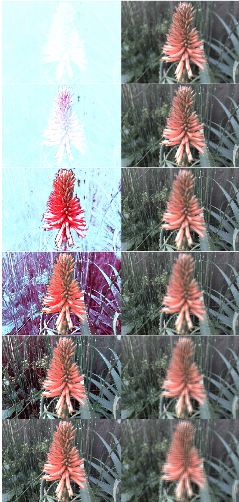
Figure 4.3: Visualization of the LSTM state at different RNN iterations (to be read from top to bottom). On the left we show the decoded memory state of the LSTM, on the right, we display the refocused 4 input views to see which depth plane is currently valid.
