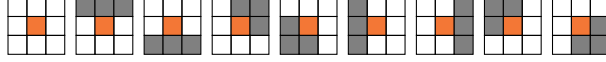
Figure 6.1: Example of angular patches in \Omega for a light field of 3 \times 3 views. The orange color corresponds to the reference view (s_c, t_c) so the angular patches are equal to 1 at this position. White positions corresponds to visible rays, so its value is equal to 1, and grey positions are equal to 0. The leftmost patch assumes the ray is visible in all views. Other patches correspond to partial visibility.
