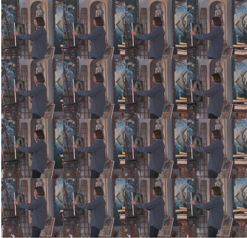
Figure 2.2: Example of a light field captured with a camera array. Because a camera array multiplexes the spatial dimension into the angular dimension, the result is a matrix of views with different viewpoints.
