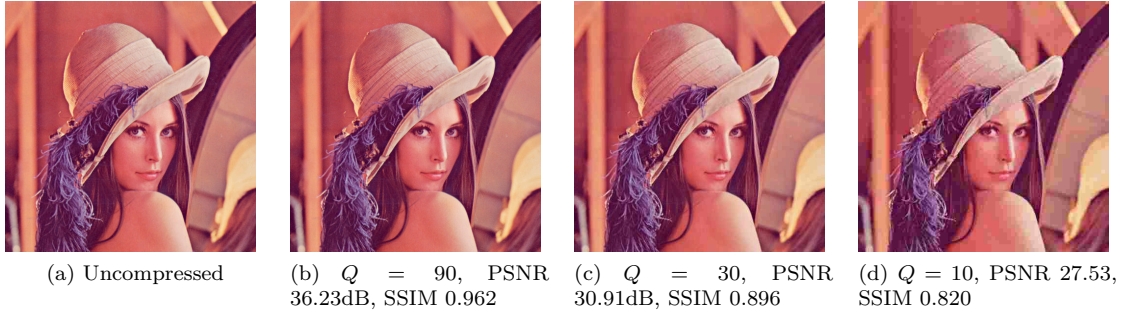
Figure 2.9: Example PSNR and SSIM values for the test image Lena encoded with JPEG ( libjpeg [16]) at various quality levels ( Q ).
