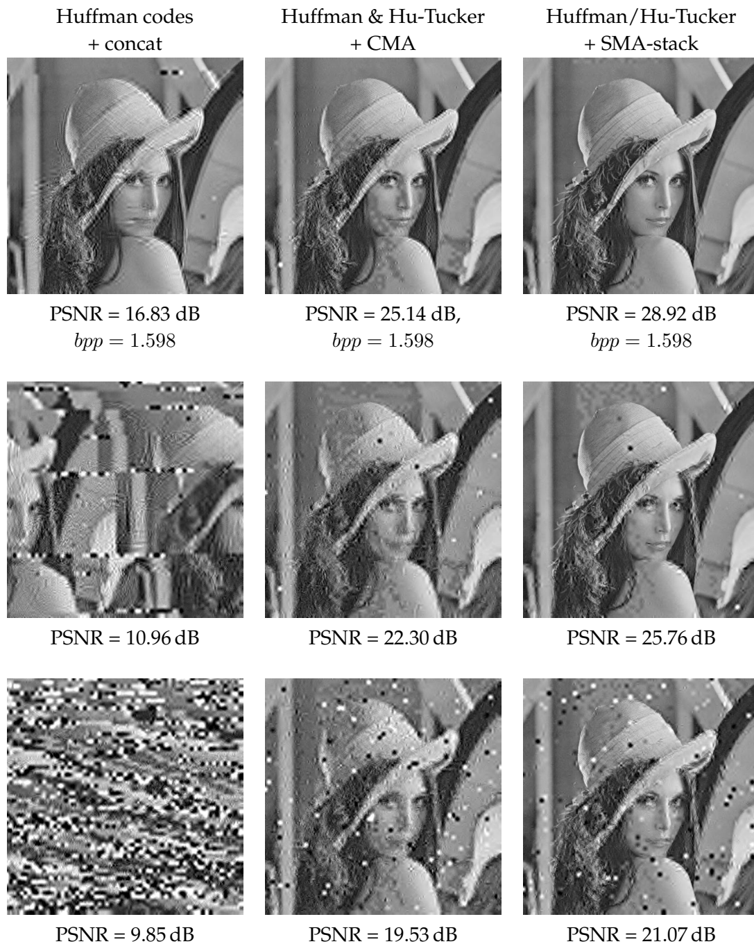
FIG. 6.11 – PSNR performance and visual quality obtained respectively with concatenated Huffman codes and two transmission schemes using Hu-Tucker codes for low subband and Huffman codes for high subbands. These schemes use respectively the CMA algorithm and the SMA-stack algorithm. The channel bit error rates are 0.0001 (top images), 0.001 (middle images) and 0.01 (bottom images).
